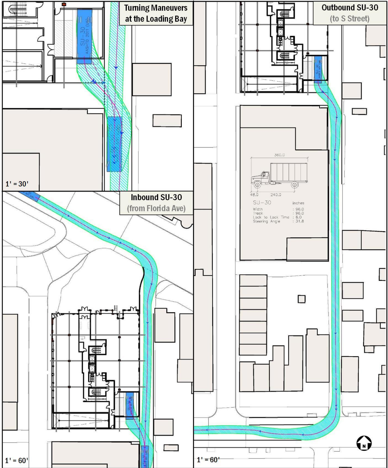
Figure 9: 30' Truck Maneuverability Diagram
